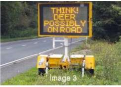
The type of dynamic sign shown in Image 2 (centre) is powered using a solar panel above, and thus does not necessarily require mains supply where this would be costly to provide. They also tend to have options to be active continuously or only at certain times of the day and year when risk is considered greatest, as well as facility for automated recording of times and frequency of activation to assist, e.g. with monitoring speed reduction achieved over time.
